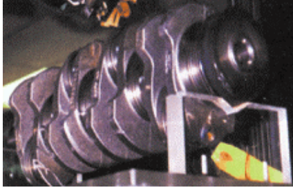
X-ray mapping measures residual stress in a crankshaft at Windsor Lab. Dynamometer tests will be done on parts with and without cryogenic treatment.
