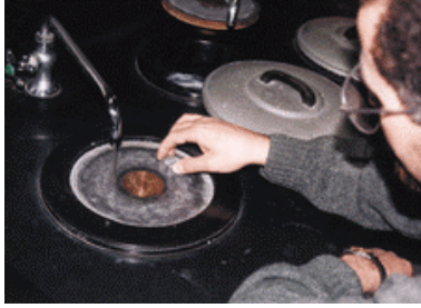
A technician polishes discs of 4340 and 9310 steel alloy, comparing conventional quenching results and quenching followed by cryogenic tempering.
